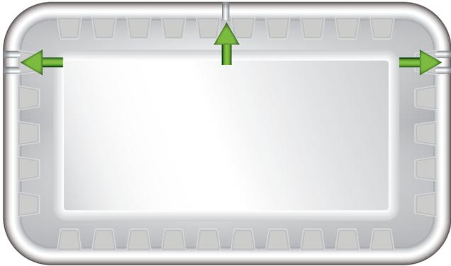
Remove the lid from the SuperPonic XL12 system and set it aside for now. Notice the channels located on the rim of the Reservoir. These channels will be for the placement of your Air Pump Tubing and Water Pump power cord.
