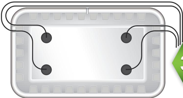
Connect the Air Pump Tubing to the end of the Air Stones. Arrange the tubing into the channels located on rim of the Reservoir.
